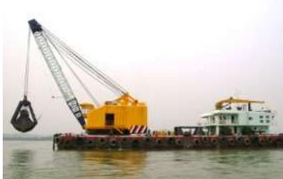
A barge with a yellow crane and a large black grabber bucket, positioned in a body of water.                                                                 |
